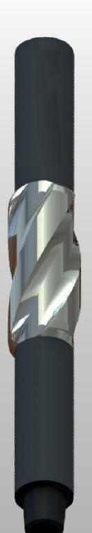
The design of the CTX Drift Sub gives 360° cover and allows for maximum fluid by-pass with its aligned fluid channels during drilling, wellbore clean-up & pre-completion running operations. The CTX Drift Sub is designed to be run with the Hi-Pro (Non-Rotating) casing scraper ahead of the drift sub to remove any residual drilling fluid, scale, cement, perforation burrs and other foreign material from the ID of the casing while RIH and reciprocating the string.
